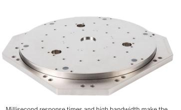
Millisecond response times and high bandwidth make the WP-Z-120A wafer positioning system ideal for applications where high throughput is essential. The stage is designed to hold 300 mm (12") wafers and delivers exceptional performance with loads of up to 8 kg suitable for heavy wafer chucks.
