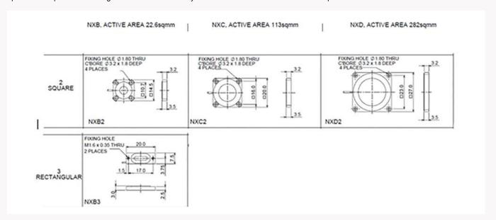
UHV variants are typically good down to 10-9Torr and can be baked out at up to 100°C for two days prior to installation. Custom Sensors
