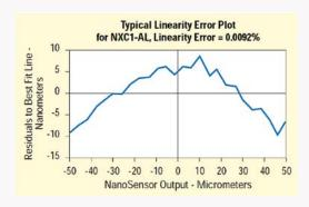
The graph shows the linearity error of a NXC2-AL sensor, in this example it is <0.01%. This is achieved without electronic compensation. . Below 0.1%, linearity error is dominated by the parallelism of the mounting surfaces. For the highest linearity choose a large gap sensor and measure over a small part of the full range. For example using NXC2-L sensor over 100um of the 500um calibrated range will give <0.005% linearity.
