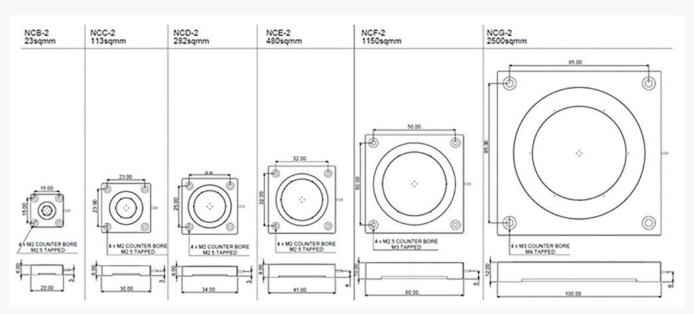
Typically good to 10<sup>-10</sup>Torr and can be baked out at up to 180°C for two days. Other shapes can be produced on request.
