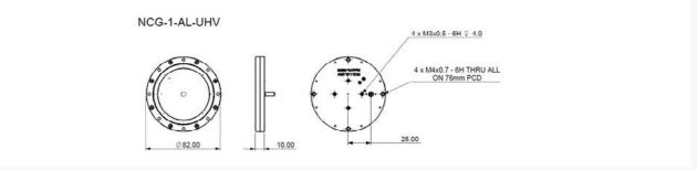
Typically good to 10<sup>-10</sup>Torr they can be baked out at up to 180°C for two days.
