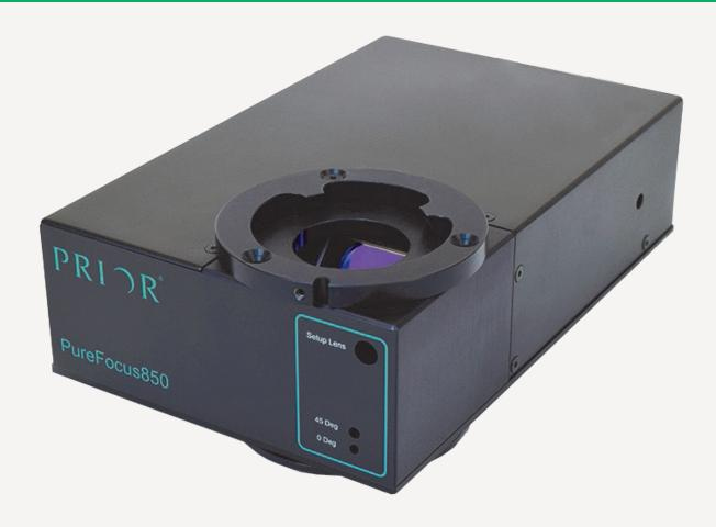
Prior Scientific's PureFocus850 combines advanced optics and intelligent in-built microprocessing to provide a real time focus system for infinity corrected optical systems. A motorized offset lens allows real-time adjustment of the imaging depth into the sample, continuously holding the precise distance between imaging focal point and a reference boundary of choice.
