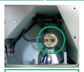
Plug the data connector into printed circuit board and replace the lamp access panel as shown above.
