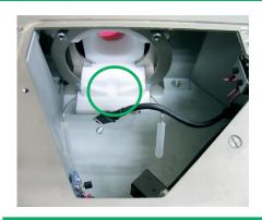
The bulb slots in with the wire into the groove (circled). Connect rear power connector
