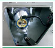
Lift springs and secure lamp in place.
